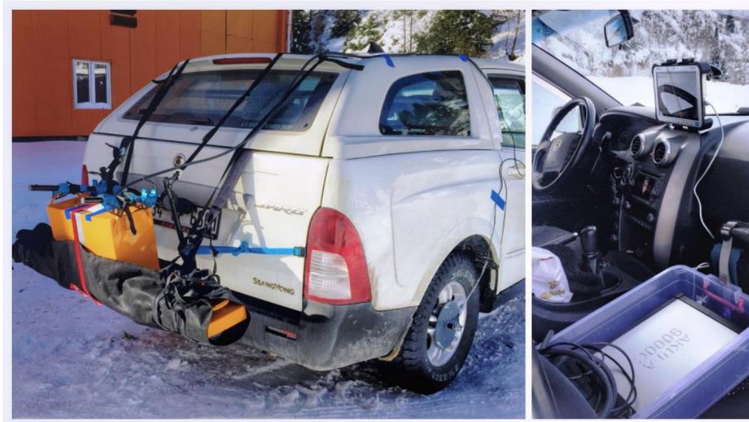
Figure 5.12 Ground Penetration Radar (GPR)/Structure Radar
